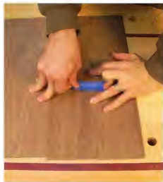
Veneer tape with a kick. Stretch tape over a veneer joint, then as the tape shrinks back, the butted veneers come together tight and secure.
